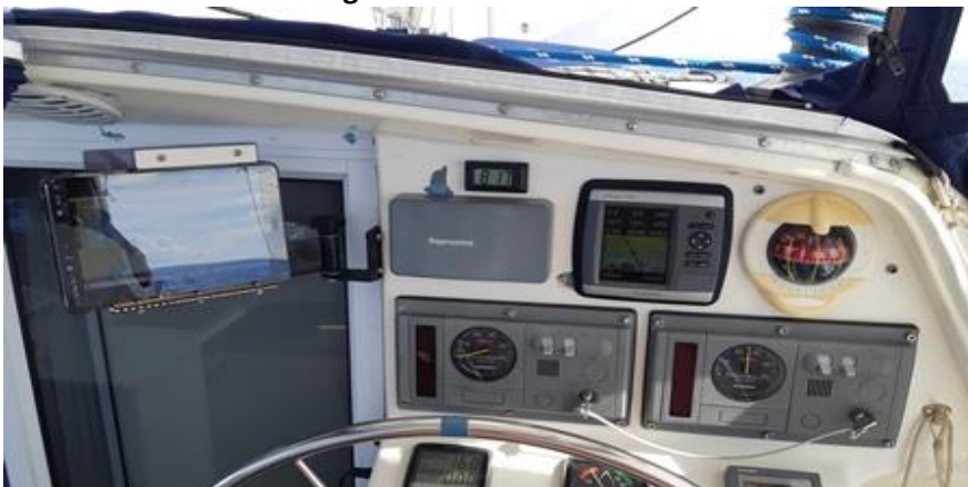
Soggy Paws Helm Station with Garmin 526S Chart Plotter On Right and Asus Tablet on Left
